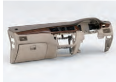
Automobile instrument panel made of polypropylene
