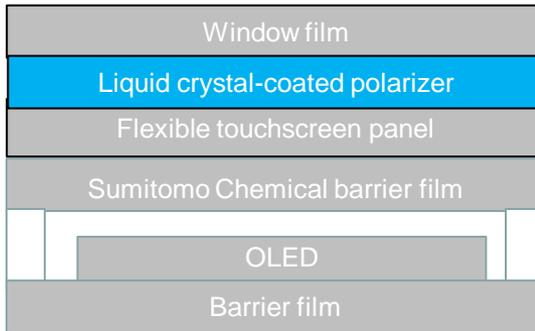
Adding characteristics of low thickness, flexible components while maintaining the fundamental characteristics of anti-reflective materials
