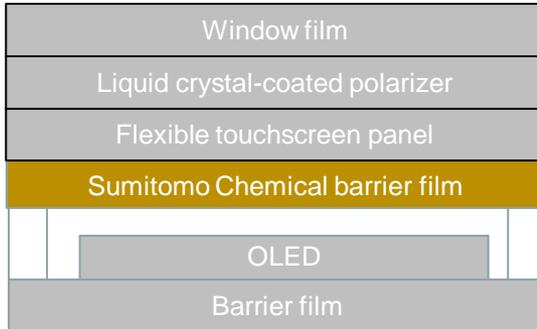
Achieving both high water vapor resistance and flexibility. Broader substrate selection, which can be applied to a variety of uses.
