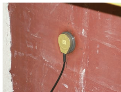
Fig. 19 The condition of FOD sensor installation on the vertical reactor
