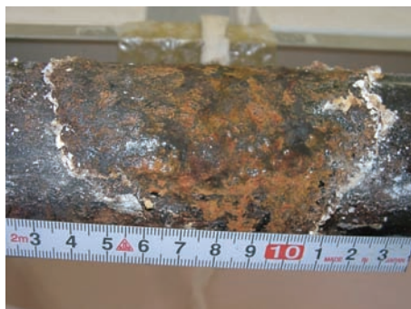
Fig. 8 Corrosion of piping (1st monitor: 11/2007)
