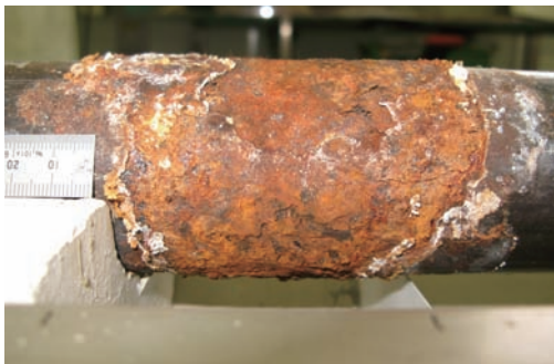
Fig. 13 Corrosion of piping (3rd monitor: 03/2008)
