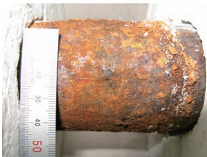
Fig. 11 Corrosion of piping (2nd monitor: 01/2008)
