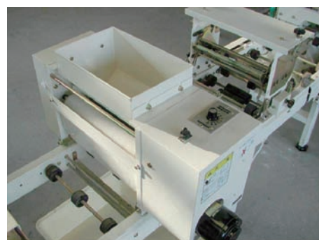
Fig. 14 Feed hopper unit for applying pesticide granules onto nursery box
