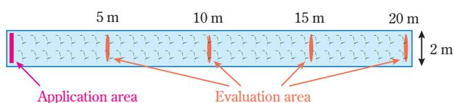
**Fig. 11** Schematic diagram of the field spreading test
