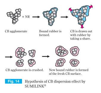
ing on the type of CC agent during the CC agent-mixing process (see **Fig. 8**, Process A), the decrease of the Payne effect and the increase in bound rubber were observed, suggesting the possibility that bound rubber may contribute to CB dispersion.
