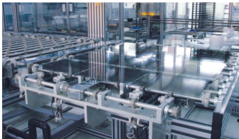
Automated, state-of-the-art color filter production facility processes glass plates for high-tech fifth-generation liquid crystal displays.
