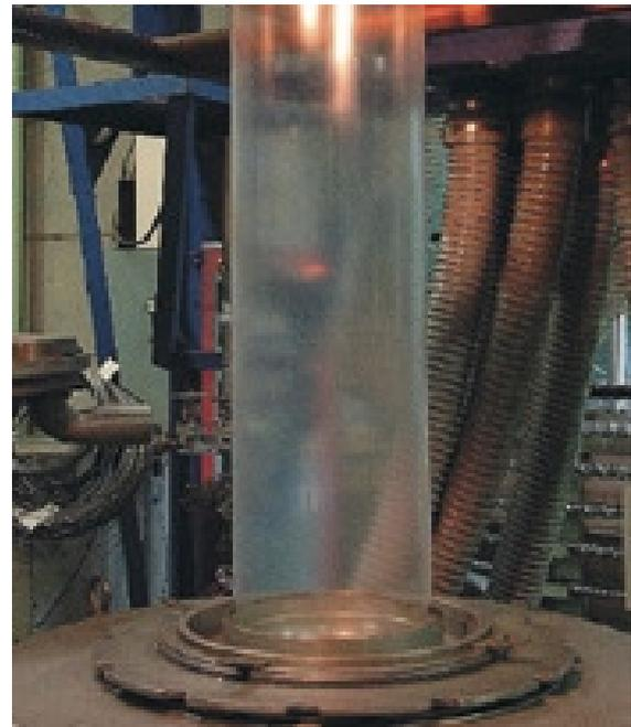
Fig. 2 Lay-flat Film of A-12 in Purging
