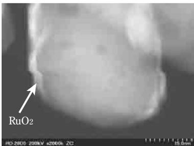
**Fig. 7** FE-STEM image of RuO<sub>2</sub>/rutile-TiO<sub>2</sub> catalyst<sup>12)</sup>
