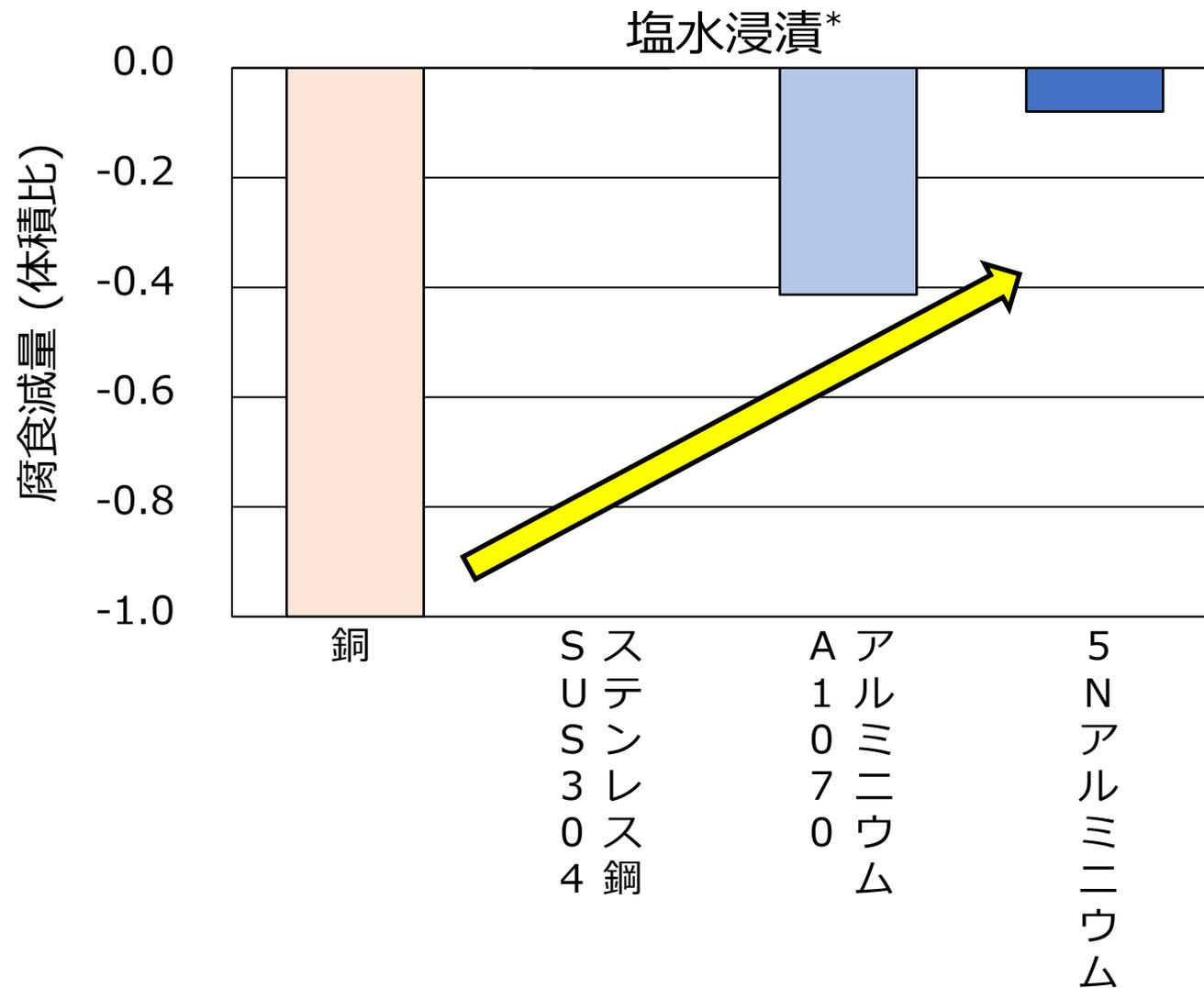
\* 3.5%NaCl aq., 酢酸でpH=3に調整, 72hr浸漬
