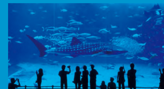
Large aquarium panel made of methyl methacrylate
