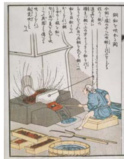
Drawing of nanban-buki copper processing from Kodo Zuroku, a pictorial booklet about copper production issued by the Sumitomo Family at the beginning of the 19th century (Source: Sumitomo Historical Archives)
