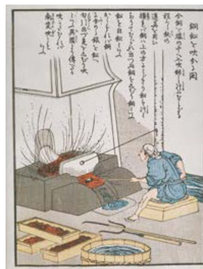
Drawing of nanban-buki copper processing from Kodo Zuroku, a pictorial booklet about copper production issued by the Sumitomo Family at the beginning of the 19th century (Source: Sumitomo Historical Archives)
