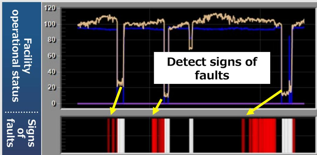
Use machine learning to detect signs of facility faults and put out an alert
