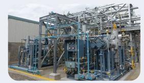
Pilot facilities manufacturing methanol from CO<sub>2</sub>
