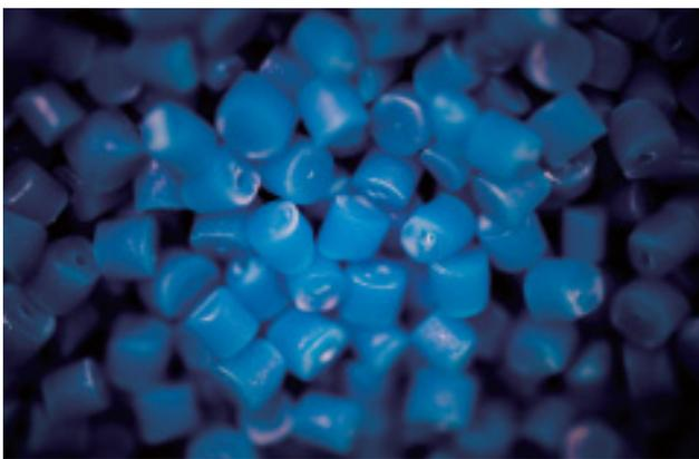
Polyethylene pellets for OLYSET® Net
