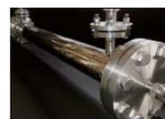
A CO<sub>2</sub> separation membrane module
