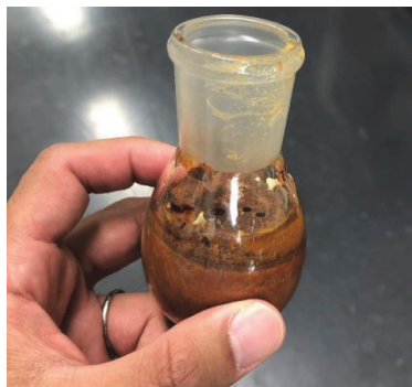
Fig. 9 Solidification of the reaction mixture during the oxidation step
