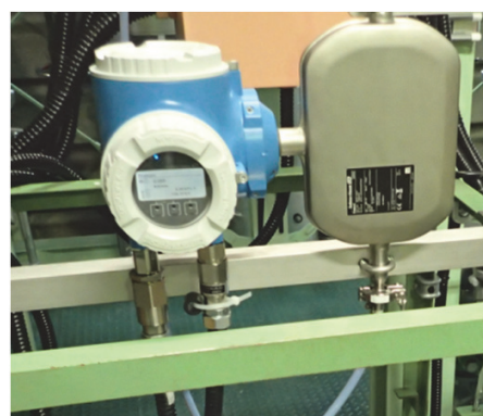
Fig. 18 Endress+Hauser, Proline Promass A 300, coriolis flow meter
