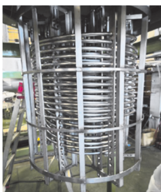
Fig. 17 corrosion-resistant and heat-resistant alloy flow reactor (inner diameter 10 mm)
