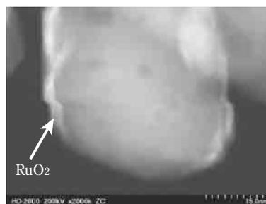
**Fig. 7** FE-STEM image of RuO<sub>2</sub>/rutile-TiO<sub>2</sub> catalyst<sup>12)</sup>
