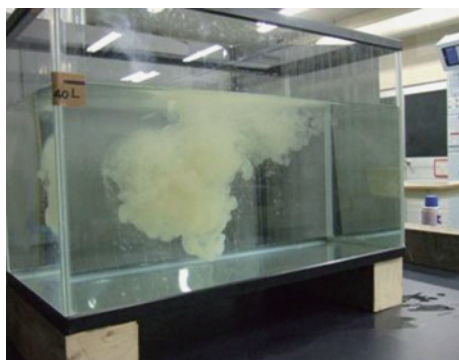
Fig. 16 Dispersibility of PIXIO®DF in water several tens of seconds after treatment
