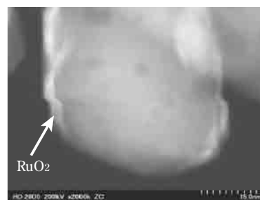
Fig. 7 FE-STEM image of \text{RuO}_2 /rutile- \text{TiO}_2 catalyst 12)
