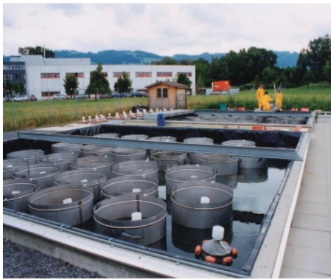
Fig. 4 Photograph of the test system (invertebrate mesocosm)
