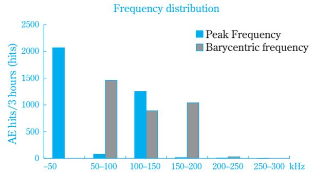
**Fig. 27** Frequency distribution of AE obtained before removing rust
