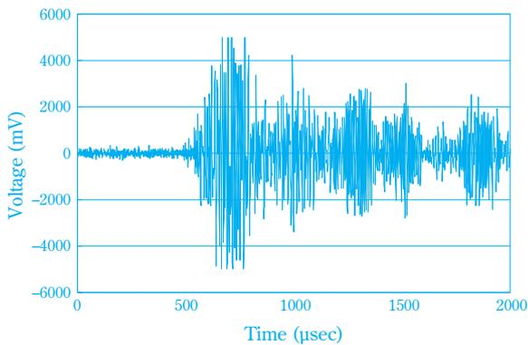
**Fig. 26** Representative Waveform of AE obtained from mock-up piping
