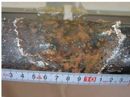
**Fig. 8** Corrosion of piping (1st monitor: 11/2007)
