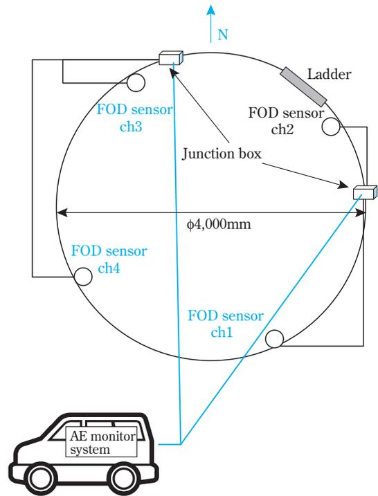
**Fig. 18** The position of FOD sensor installation and wiring for signal cable
