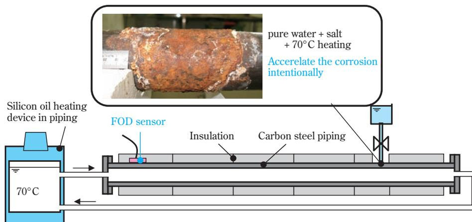
**Fig. 6** Mock-up piping for CUI inspection investigation
