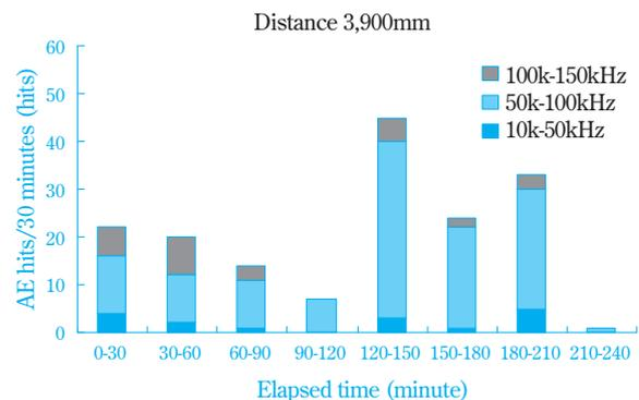
**Fig. 12** AE hits by corrosion progress at 3,900mm
