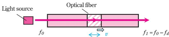
**Fig. 3** Model of Doppler effect of optical fiber
