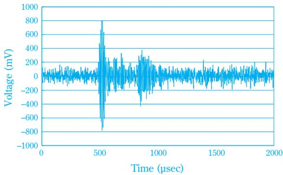
**Fig. 25** Representative Waveform of AE obtained after removing rust
