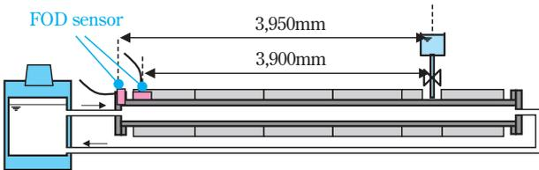
Fig. 14 The position of FOD sensor installation
