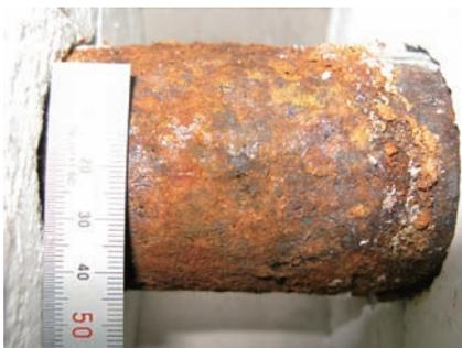
**Fig. 11** Corrosion of piping (2nd monitor: 01/2008)
