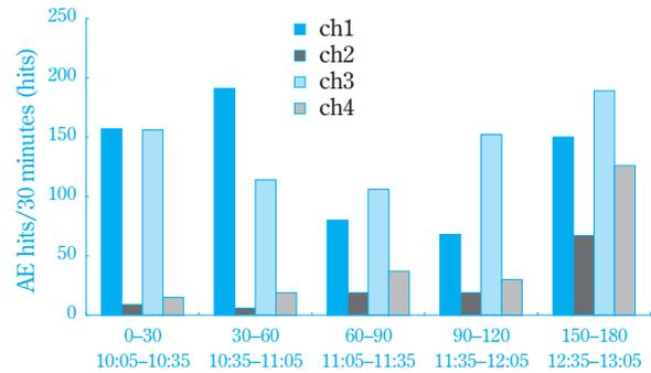
**Fig. 22** AE hits/30 minutes before removing rust
