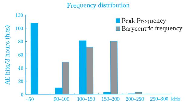
**Fig. 28** Frequency distribution of AE obtained after removing rust
