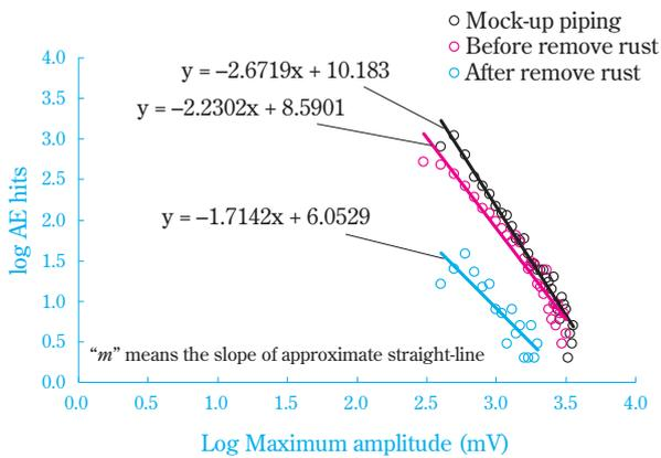
**Fig. 31** Comparison by  $m$  value (Shape parameter)
