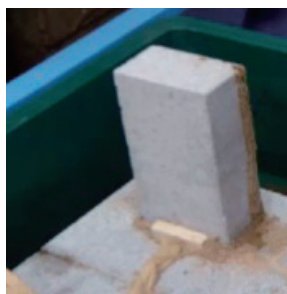
Fig. 9 Mud tubes built on an untreated concrete block one week after installation
