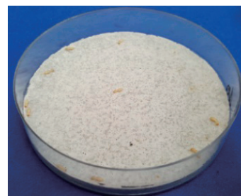
Fig. 6 Concrete plate contact test method
