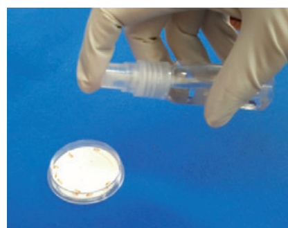
Fig. 12 Direct spray test method
