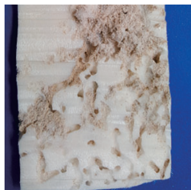
Fig. 20 Heat-insulating material damaged by termites
