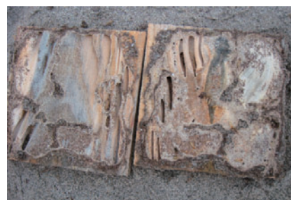
Fig. 4 Wood block damaged by termites on untreated soil
