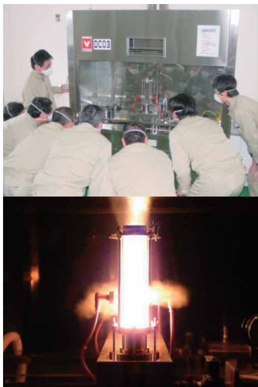
Fig. 10 An experiment of dust explosion
