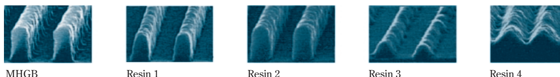
Fig. 9 Comparison of 150nm 1 : 1 L/S of resists
