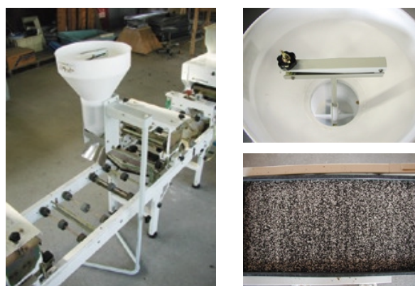
Fig. 5 An apparatus for granule application to nursery box
