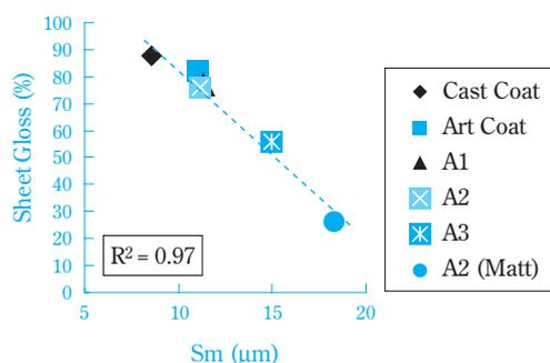
**Fig. 2** Surface Roughness ( $S_m$ ) vs. Sheet Gloss
