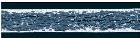
**Fig. 1** Cross Section of Coated Paper (SEM Image)
