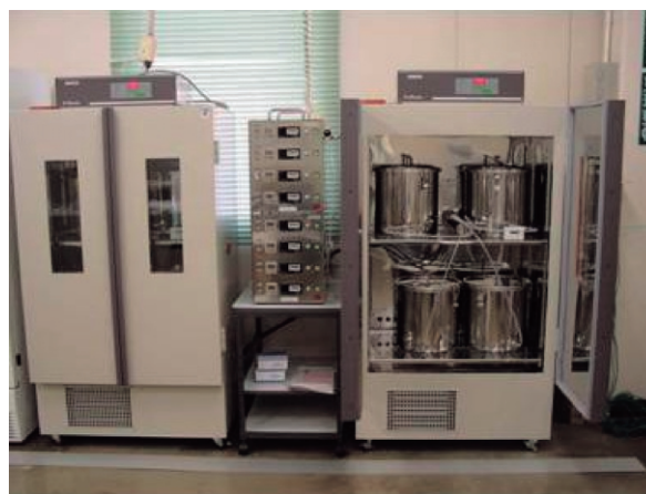
Fig. 2 JIS small chamber system (chamber volume : 20L)
