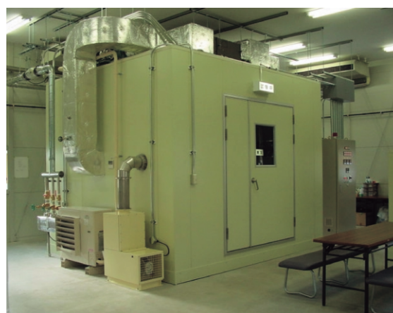
Fig. 3 Large chamber system (chamber volume: 20\text{m}^3 )
