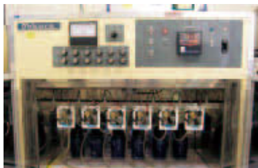
A device at the EHSL for testing biodegradability
