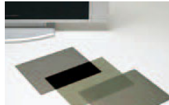
Polarizing film indispensable for LCD TVs
