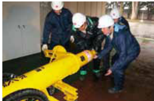
Putting a chlorine cylinder into a case
