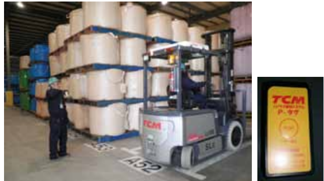
Forklift with a mounted panoramic detection system and alarm tag
