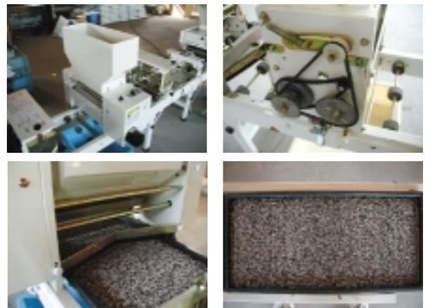
**Fig. 9** An apparatus for granule application to nursery box (Suzutech: type SDP-33S)
