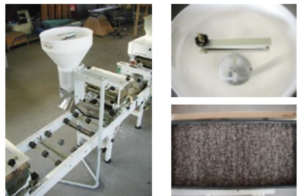
**Fig. 10** An apparatus for granule application to nursery box (Bizen: type SK-10)
