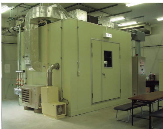
Fig. 3 Large chamber system (chamber volume: 20m 3 )
