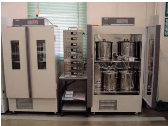
Fig. 2 JIS small chamber system (chamber volume : 20L)
