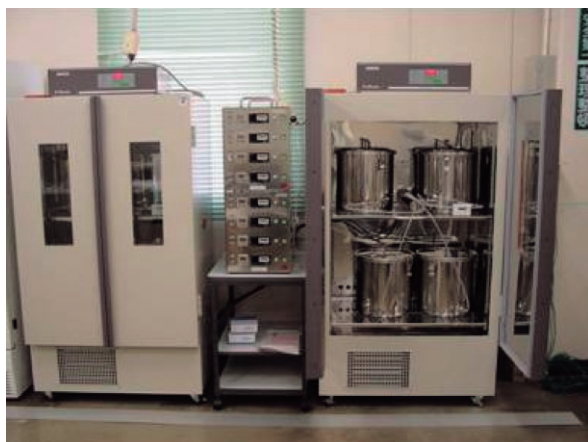
Fig. 2 JIS small chamber system (chamber volume : 20L)
