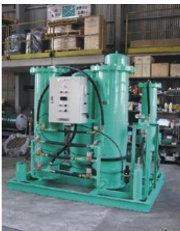
**Fig. 3** N<sub>2</sub> PSA Unit
