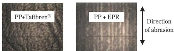
Test method : JASO-M-403-11B (Flat surface abrasion tester)
