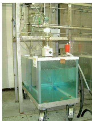
**Fig. 3** An experimental apparatus for bioconcentration test
