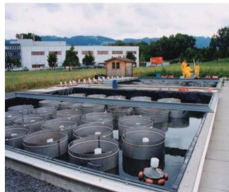
**Fig. 4** Photograph of the test system (invertebrate mesocosm)
