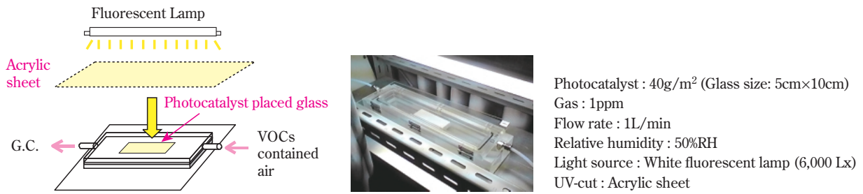
Fig. 10 A picture and an illustration of the experimental setup for photocatalytic decomposition of VOCs using a flow type reactor under a fluorescent lamp irradiation
