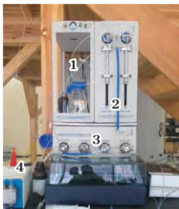
1: Organizer 2: HPD LC-SPE-NMR Dispenser 3: ACE LC-SPE-NMR Interface 4: Dilution pump
