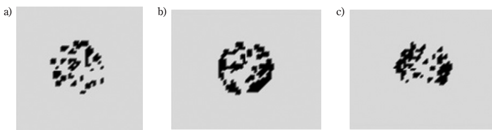
Fig. 2 The cross-sections of a cluster in three orthogonal planes; a) xy-plane, b) yz-plane, c) zx-plane. Black dots show the positions of inclusions.
