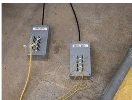
Fig. 20 Connection of 4ch FOD sensor to junk BOX
