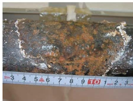
Fig. 8 Corrosion of piping (1st monitor: 11/2007)
