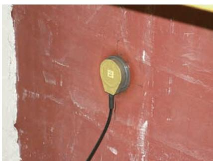
Fig. 19 The condition of FOD sensor installation on the vertical reactor
