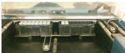
SPE unit (96 cartridges  $\times$  2)
