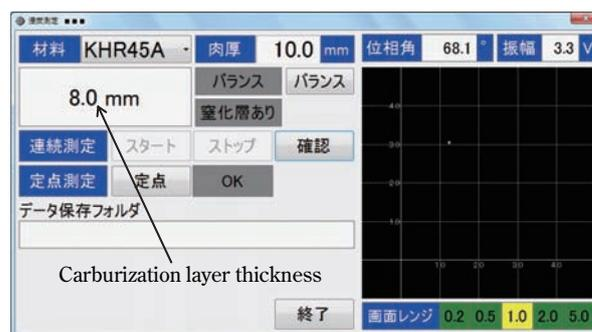
**Fig. 27** Screenshot of portable carburization measurement instrument
