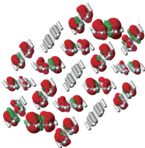
Fig. 5 Spin density calculated for isolated, first- and second-nearest-neighbor pentacenes
