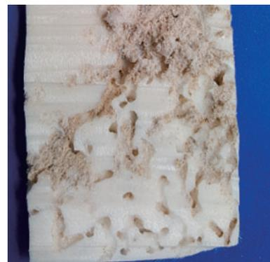
**Fig. 20** Heat insulating material damaged by termites
