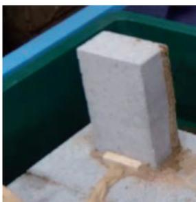
**Fig. 9** Mud tubes built on untreated concrete block in one week after installation
