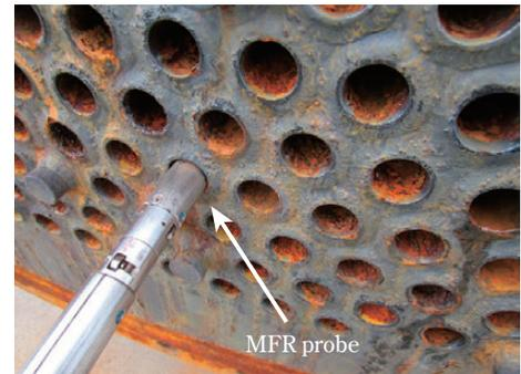
**Fig. 8** Inspection status of heat exchanger by MFR
